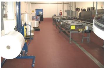
Stonclad UT replaced an unsafe, failing epoxy floor in Cold Springs Brewery's batching rooms.
