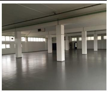
Stonclad GS, a troweled epoxy mortar system, provides this production facility with superior impact, abrasion and chemical resistance.
